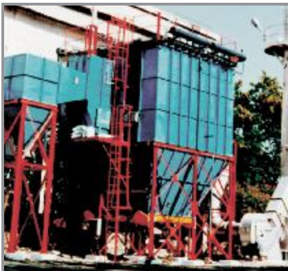
A typical casing entry bag filter with spark arrestor for Metalurgical Application
